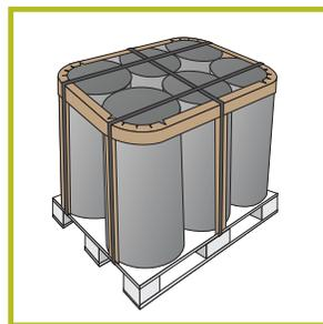
Perforated W-profile with a suitable step can flexibly help to protect round and straight edges.
