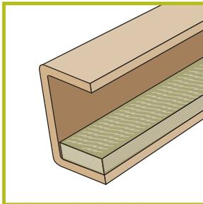
The padding glued on the edge of the U-profile helps to protect the protruding parts of goods.
