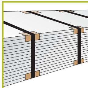
Edge protectors protect packaged goods from pressure caused by packing tape.
