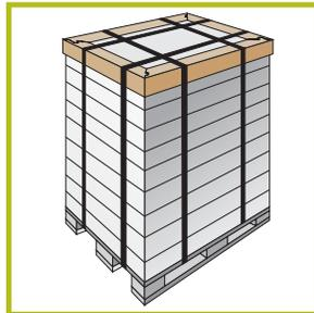
Edge protectors can also be used for protecting horizontal edges where necessary.
