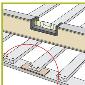
I-profile is useful in levelling and adjusting processes.
