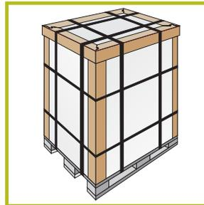
Simultaneous use of vertical and horizontal edge protectors provide particularly firm protection for the goods.
