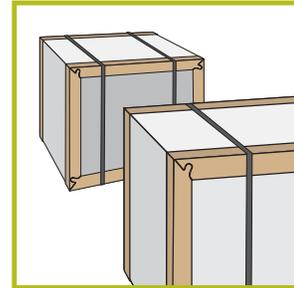
Frame profile strengthens the package and therefore enables the products to be loaded on top of each other.
