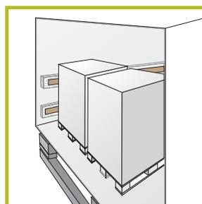
Fixed I-profiles on walls protect the goods from friction.
