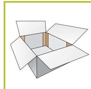
Edge protectors provide higher load tolerance and stability to cardboard box.
