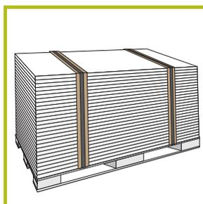
I-profile protects the surfaces against the pressure of the packaging straps.
