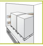
Fixed I-profiles on walls protect the goods from friction.
