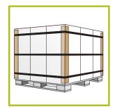
When placed in vertical position the edge protectors protect the edges of packaged goods.
