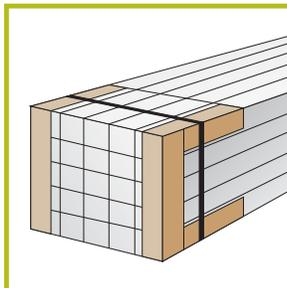
Protection of the package ends against shock and pressure caused by packing tape.
