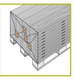
The short I-profile is usable under the cover braces in order to prevent the brace from being pulled through the cover.
