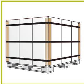
When placed in vertical position the edge protectors protect the edges of packaged goods.
