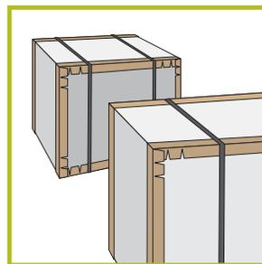
The client is able to order the necessary step density of the W-profile to protect edges and corners.
